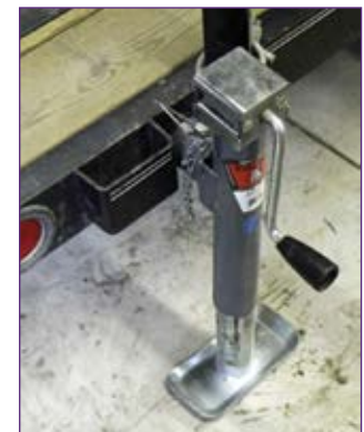
Pipe Mount Jack mounted on the frame of a trailer for stabilization or leveling.
