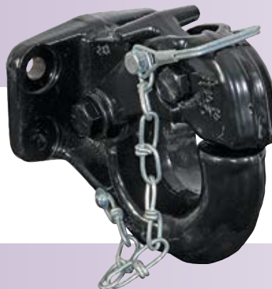
8550029 2" to 3" I.D. Drawbar - Pintle Hitch. Heavy-Duty Drop Forged Alloy Steel. Black Powder Coat Finish. Individually Boxed. 15-Ton Capacity
